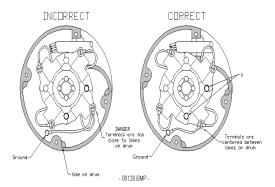
The last brush assembly--one closest to steel hub on collector ring--must be assembled on brush studs indicated by the "X" in Figure 1. NOTE: Check position of cable entry in relationship to studs marked by "X" in Figure 1. Replace subsequent brush assemblies in clockwise rotation.
