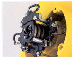
Compact 30-amp modular collector rings can handle up to 16 conductors. All brushes are spring loaded copper/graphite for positive electrical contact.
