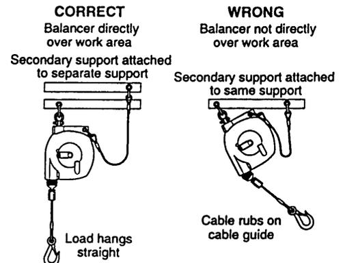
**WARNING:** To prevent personal injury, death or property damage, do not attach secondary support to same structure that supports balancer.
