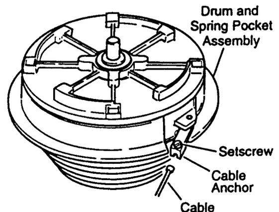
**WARNING:** To prevent serious injury, death or property damage, do not release drum lock lever (31) without installing load on tool clip. Cable and tool clip will retract rapidly.
